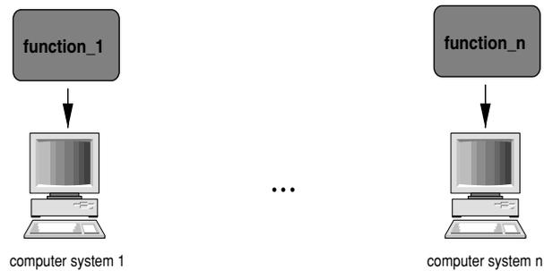
Fig. 3. Federated architectures. Each avionics function has its own fault-tolerant computers.
