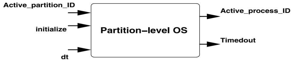
Fig. 11. Interface of the partition-level OS model.
